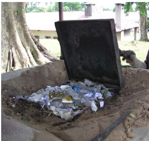
Incinerator charged with waste before lighting
