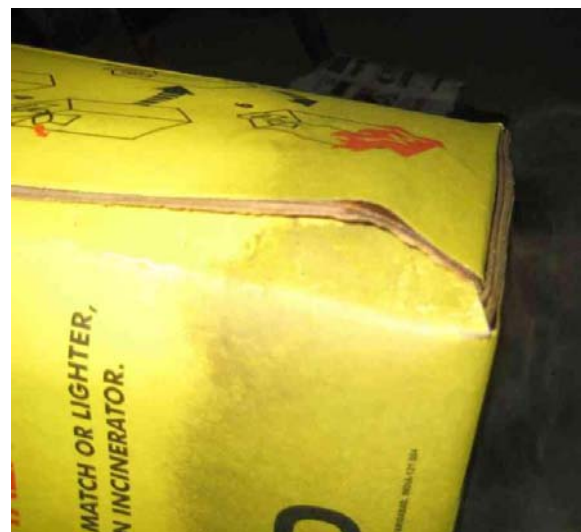
Minor wear on the glued joint
