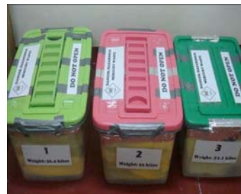
Sealed and labeled secondary container ready for storage. (Abejar-Arago, 2008)
